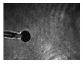
Fig. 5. The transmission type caustic image of a transparent specimen (a crack shown on the image).
