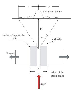
Fig. 8. The optical strain gauge.
