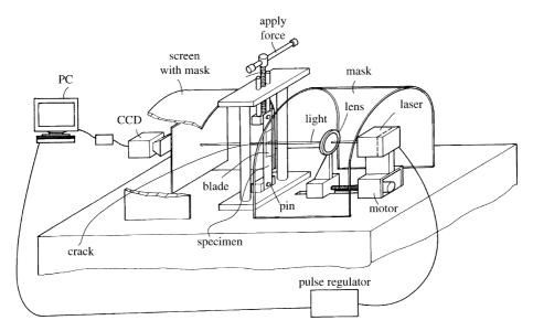
Fig. 10. The novel experimental device with modified laser shadow spot and optical strain gauge set-up.
