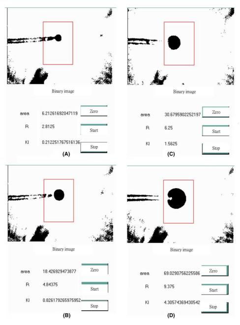
Fig. 17. (A)-(D) The images changed with the increasing of strain on an acrylic specimen.
