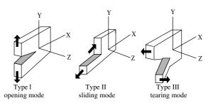
Fig. 1. The three types of the crack.
