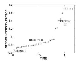
Fig. 3. The relation between time and stress intensity factor in the growth of crack.
