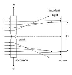
Fig. 2. The laser shadow spot.
