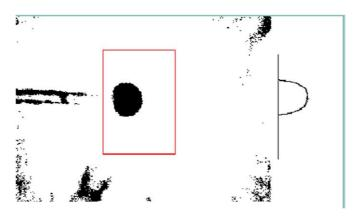
Fig. 16. The binarization image and the statistic diagram of horizontal dark spots.
