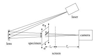
Fig. 6. The ray path of a caustic.
